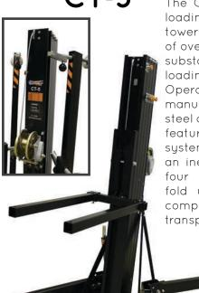
The CT-5 is a front loading telescopic tower with a height of over 21 feet and a substantial weight loading of 529 lbs. Operated via a manual winch with steel cable, the CT-5 features two safety systems, including an inertia lock. The outrigaers fold up to give a compact size for transportation.
