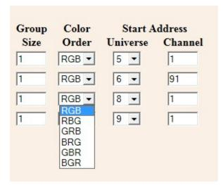
**Start Address** Each output that is marked as in use, and has a length greater than 0, is assigned a sequential block of DMX addresses. The length of this address block is (Length in Pixels) X 3, because each pixel requires 3 channels, one for each of its primary colors; red, green, and blue. Note that if pixel grouping is used the number of channels needed will be reduced accordingly.
