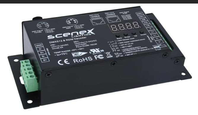
The LEDDRV5CHAN, 5 channel DMX driver is a great innovation from SceneX Lighting. It is an industrial level DMX512 & RDM controller featuring both DMX decoder and DMX master capabilities. It is easy to switch between master mode and decoder mode. With full support of the latest DMX512, DMX512(1990), DMX512-A and RDM V1.0 (E1.20 – 2006 ESTA Standard) protocols.
