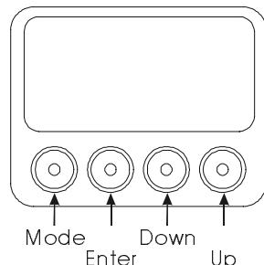
To lock or unlock the keys of the menu field press Mode+Enter+Up simultaneously.
