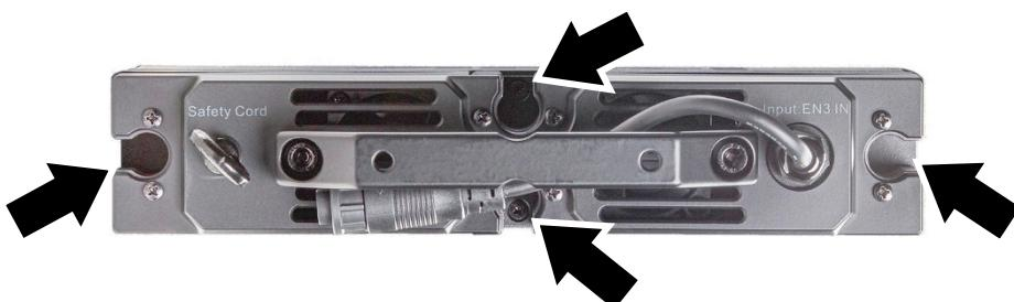
**Figure 18. Mechanical connector channels on KNV Line**
