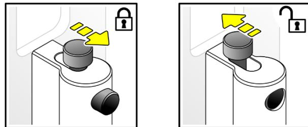
**Figure 19. Locking mechanism on KNV Line Floorstand and Brackets**
