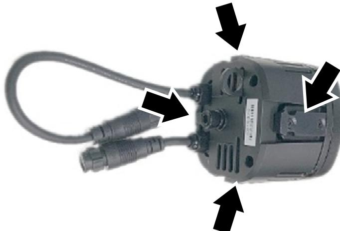
**Figure 9. Channels for Slide Connectors in KNV Dot**
