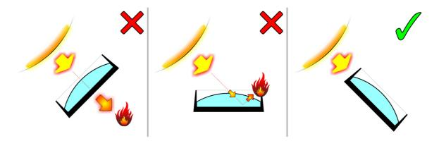
Figure 1. Avoiding damage from light sources
