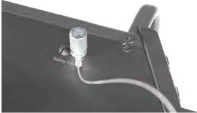
Figure 11. Optical accessory safety cable attachment
