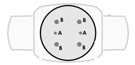
Figure 5 Mounting points in base
