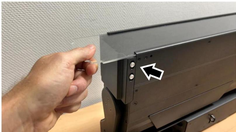
**Figure 7. Filter slide-in locks**
